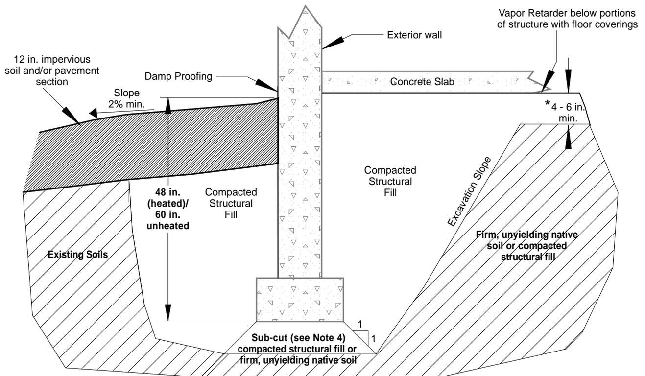
**TYPICAL FLOOR SLAB AND FOOTING DETAIL**
