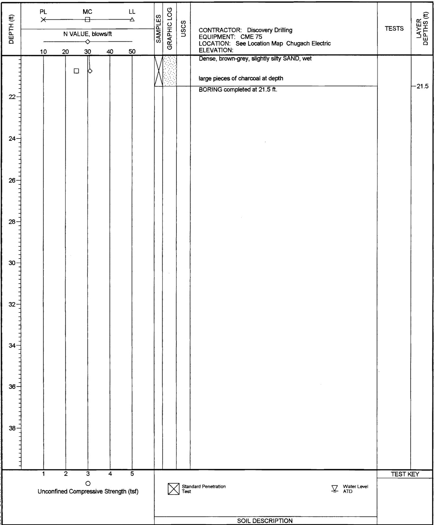
LOG OF BORING CHUGACH SUBSTATION GPJ HDEC.GDT 7/12/02 10:36
