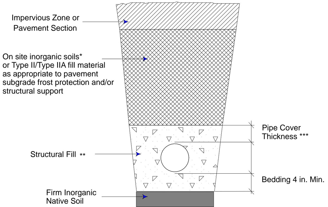
\* Inorganic soils, 95% compaction below structural fill supporting footings, streets, etc., 90% compaction in non structural support areas.
