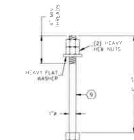
DETAIL 3 ANCHOR BOLT FOR CIRCUIT BREAKERS ASSEMBLY A81 (4 REQ'D) N.T.S.
